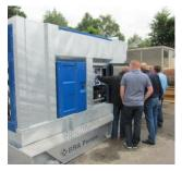
Factory Acceptance Test Extensive testing facility inhouse. FAT must be conducted formally and be witnessed by the owner and/or project manager.
